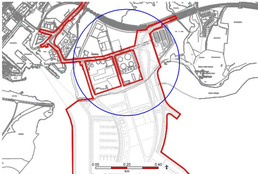
Figure 13 Tank 9 Gasoline LOC and Flash Fire: Worst Case Flash Fire Contour
